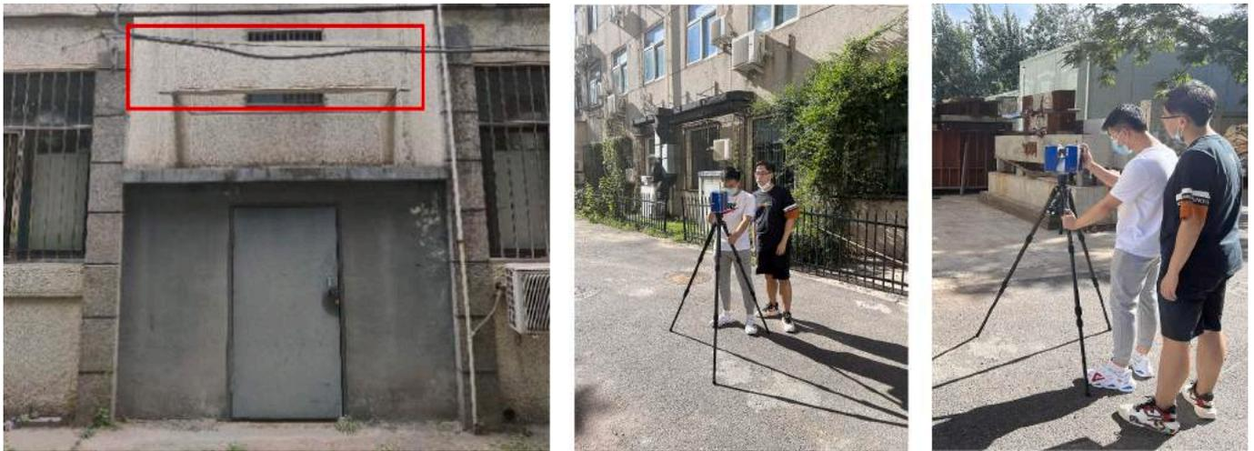
Fig. 6. Spatial details data acquisition through TLS and GNSS.
