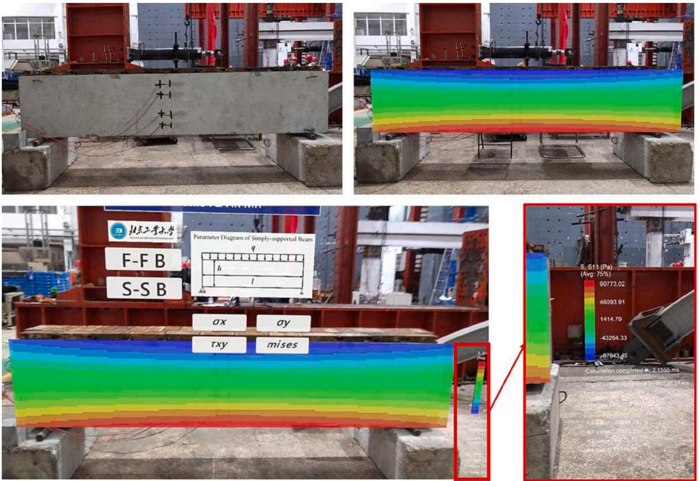
Fig. 20. In-situ application of the MR-FEA system.
